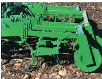
Rastra delante del rulo Herses devant le rouleau Harrow in front of the roller
